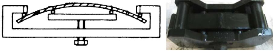
Figure 11. Four point loading.
