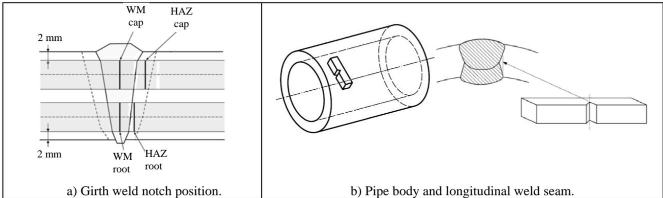
Figure 8. Specimen orientation and notches position.
