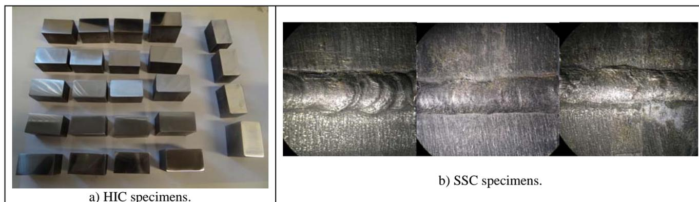
Figure 21. HIC and SSC test samples after the test.
