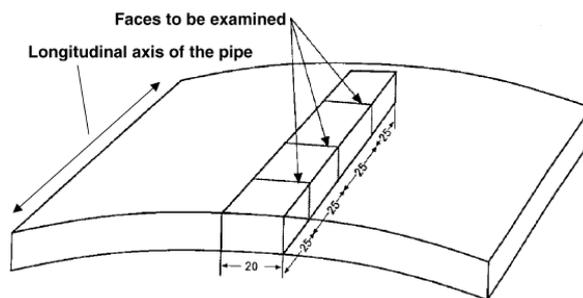
Figure 10. Orientation of test specimens.
