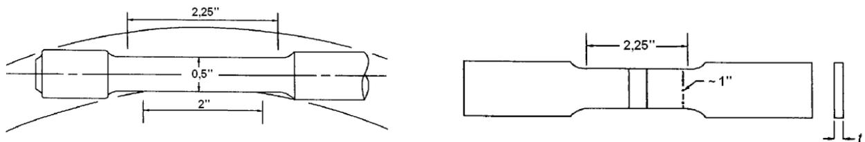
Figure 9. Tensile specimens.
