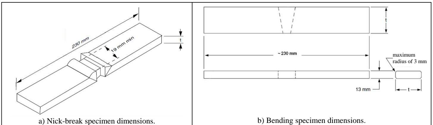
Figure 6. Nick-break and bending specimens.
