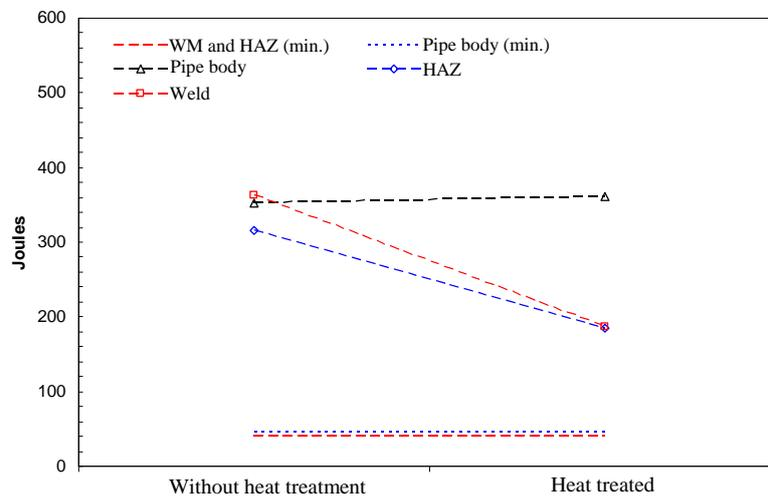
Figure 18. Pipe body and SAW longitudinal weld Charpy results.
