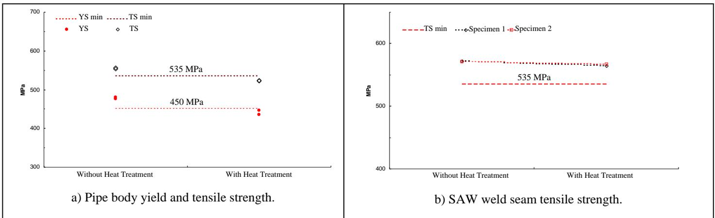
Figure 13. Yield and tensile strength results from pipe body and SAW weld seam.
