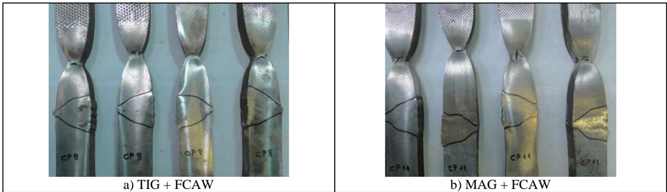
Figure 15. Tensile specimens of girth welds.
