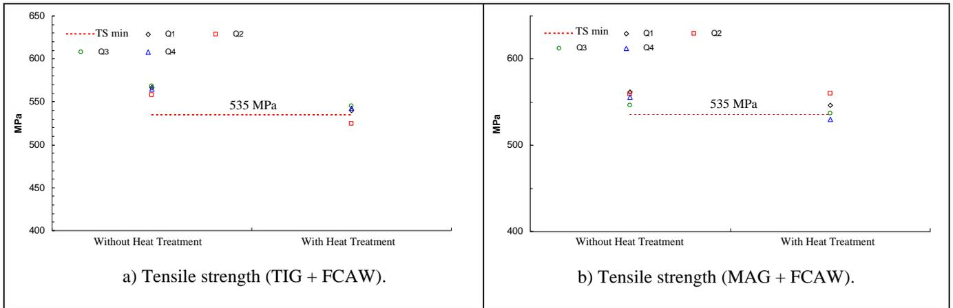
Figure 14. Tensile strength results of girth welds.
