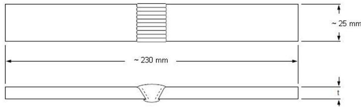
Figure 5. Tensile specimen dimensions.
