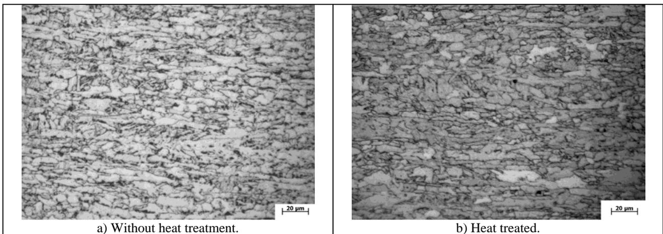
Figure 16. Microstructure before and after heat treatment.
