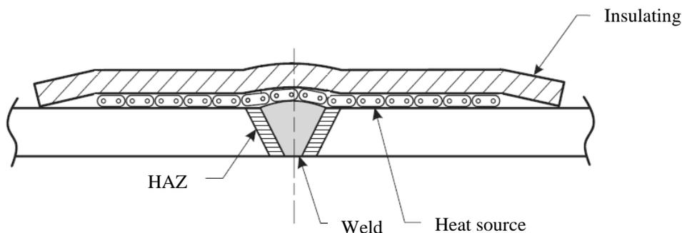
Figure 4. Electric resistance heating.
