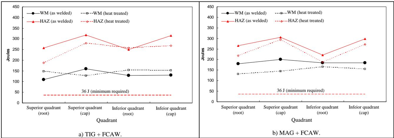
Figure 17. Charpy impact test results of girth weld.
