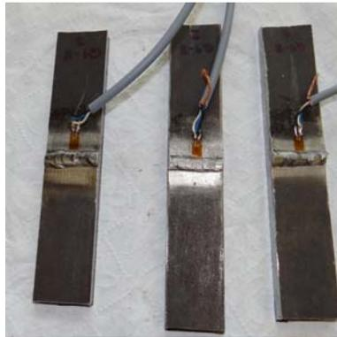
Figure 12. Girth weld specimens.
