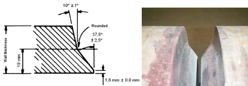
Figure 1. Bevel geometry.
